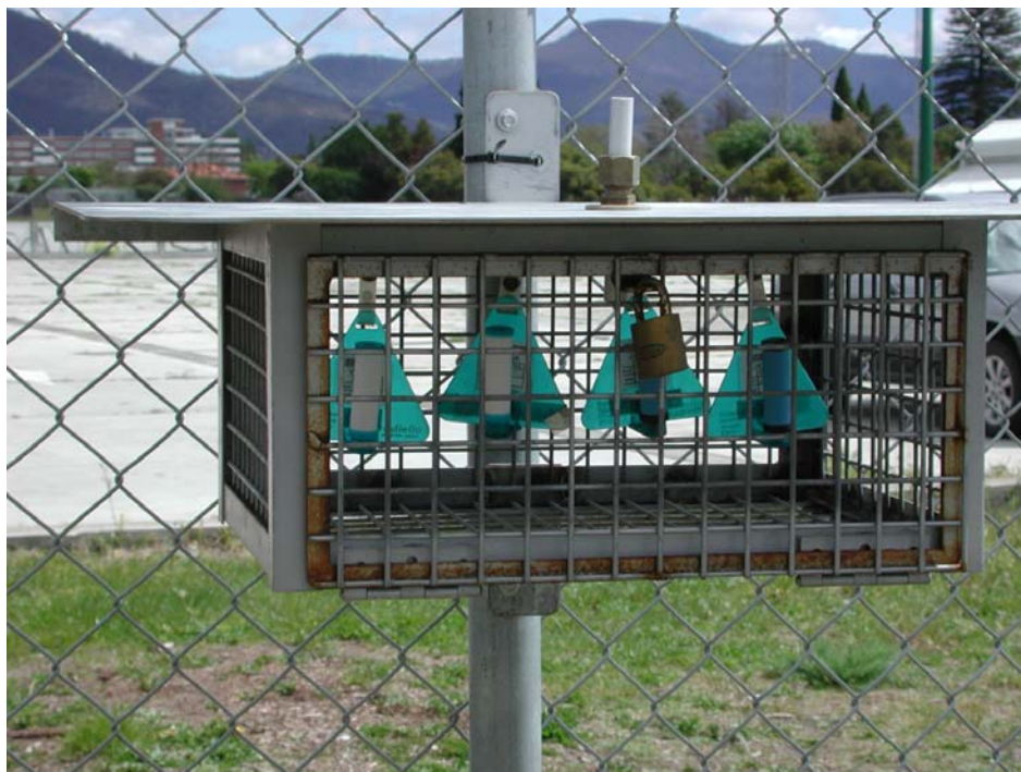
Figure 1 Radiello passive samplers deployed at New Town
