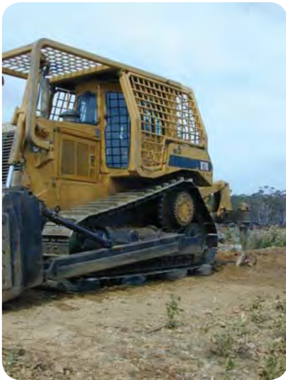
After cleaning and disinfecting, bulldozer is left to dry. Maintaining elevation with tyres allows the underside to dry. Photo courtesy of Forestry Tasmania.
