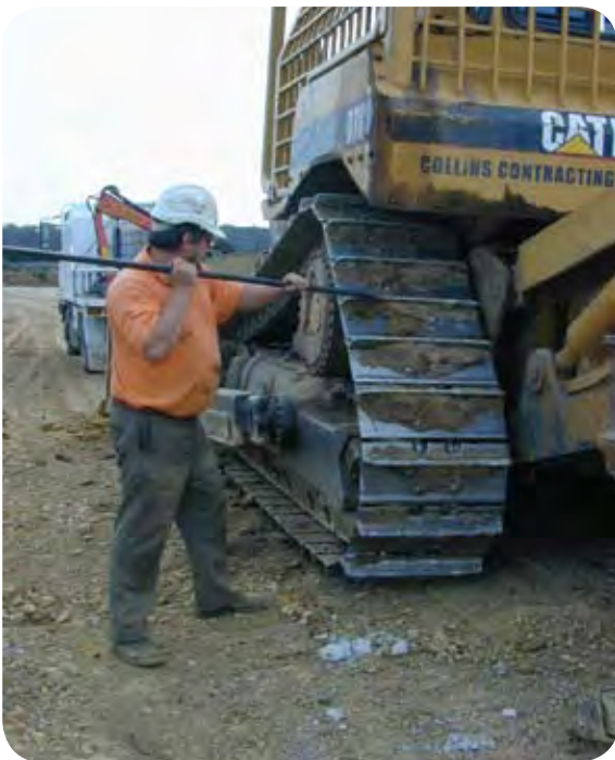
Removal of soil and dirt from bulldozer treads using crow bar. Photo courtesy of Forestry Tasmania.
