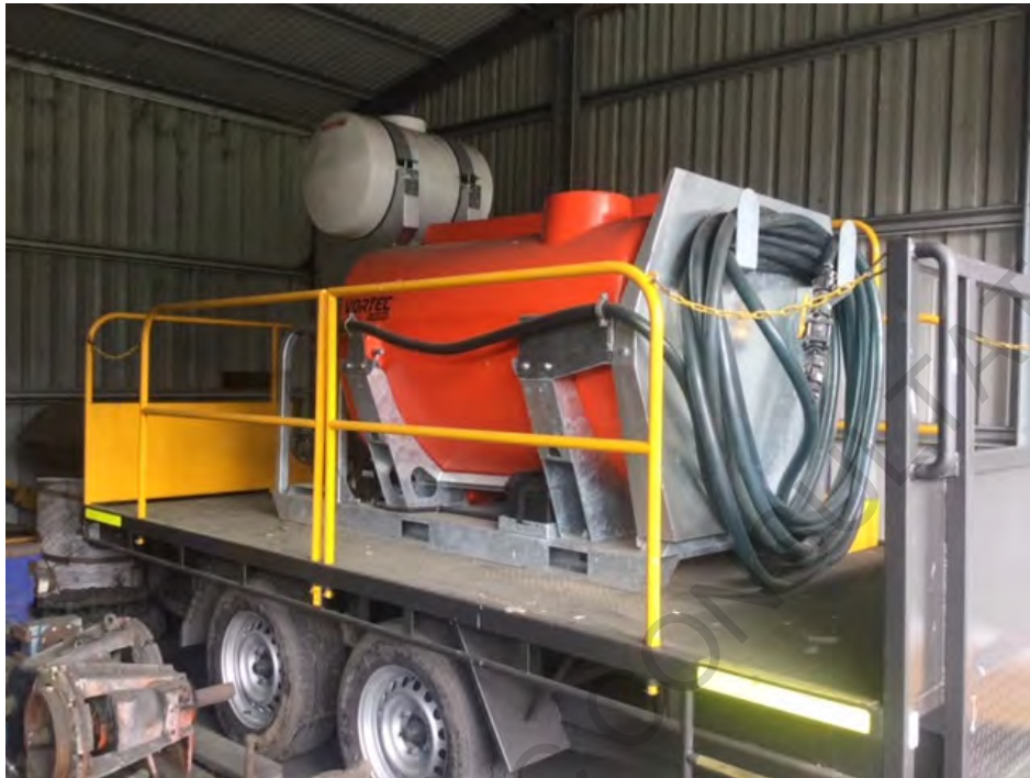
Hydromulch unit on purpose-built trailer
