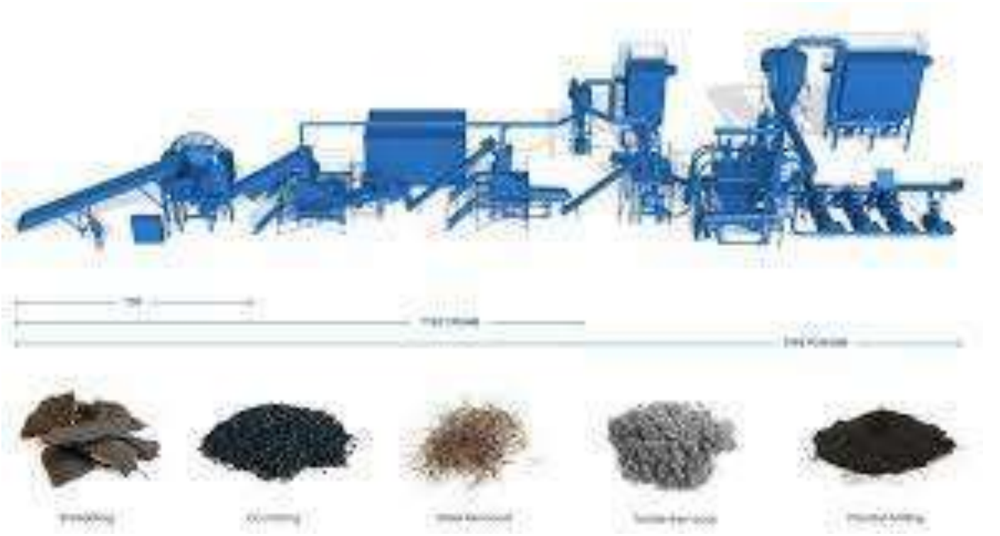
Figure 2: Shredding machine process
