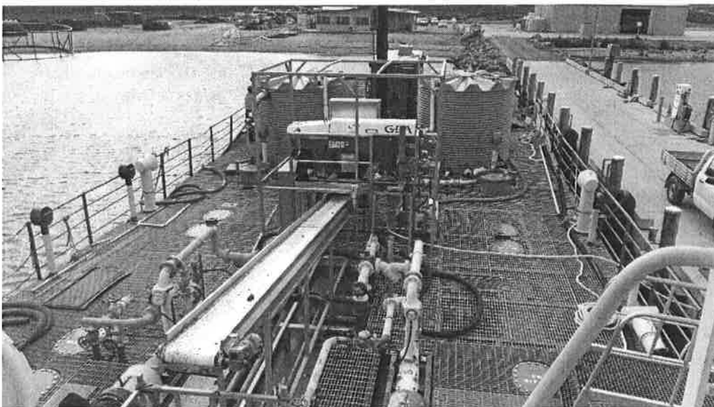
Figure 2: Foredeck of Wallaby, showing centrifuge, solids conveying and raw waste storage tanks
