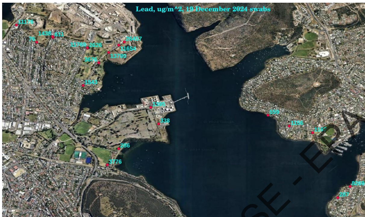
Figure 2 Lead areal-concentrations ( \mu\text{g}/\text{m}^2 ) from surface swabs on 19 December 2024
