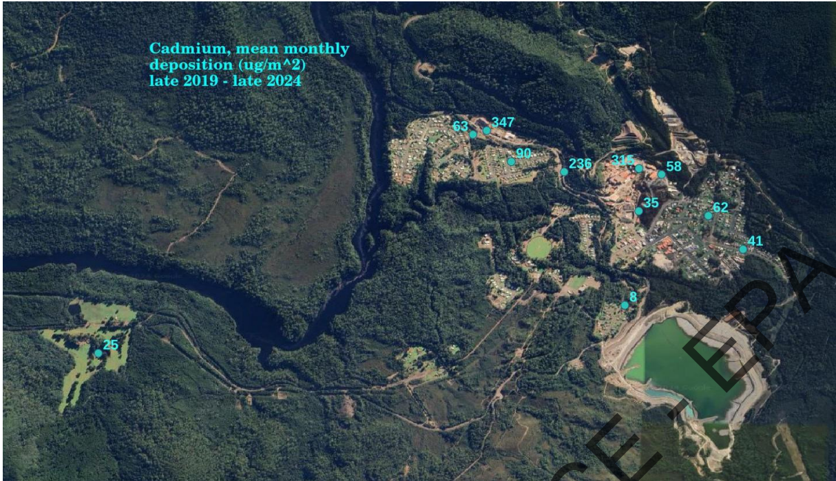
Figure 9 Mean cadmium monthly deposition rates, in \mu\text{g}/\text{m}^2/\text{month} for late 2019 to late 2024 for the I I Rosebery MMG Australia dust deposition gauges
