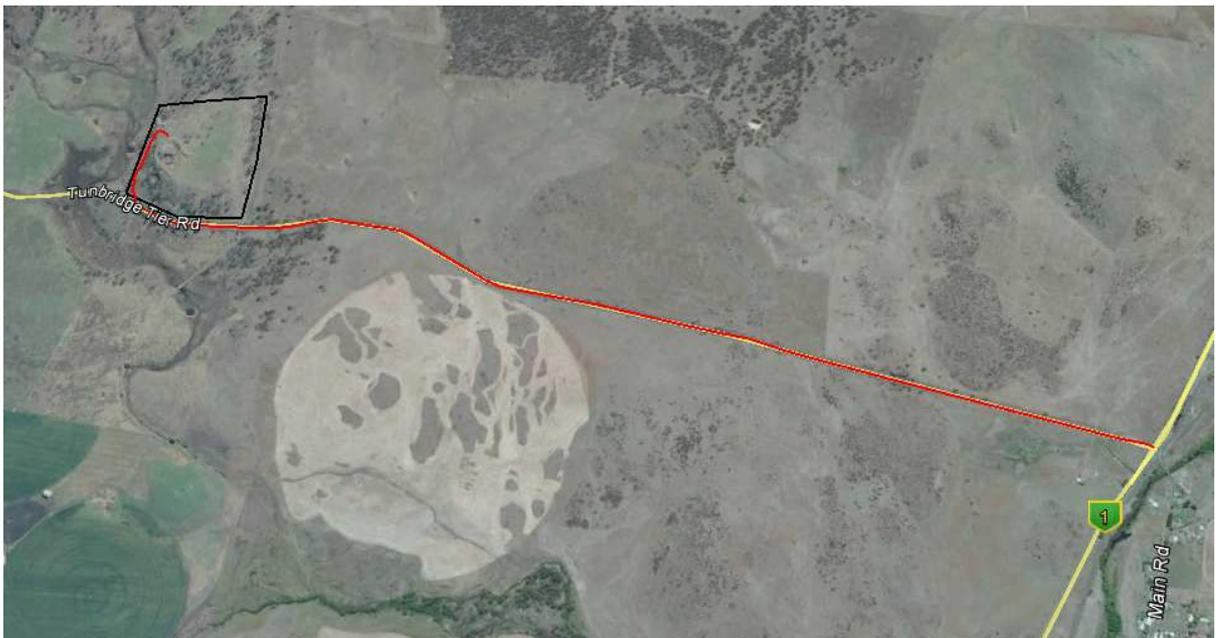
Access to the quarry is by an existing gravel driveway some 4 metres wide at the property boundary with throat width some 24 metres at the edge of seal. The driveway is generally at right angles to the road on an approach gradient of some 4%. A gravel turn in area is available on the opposite side of the road to provide for truck turns.
