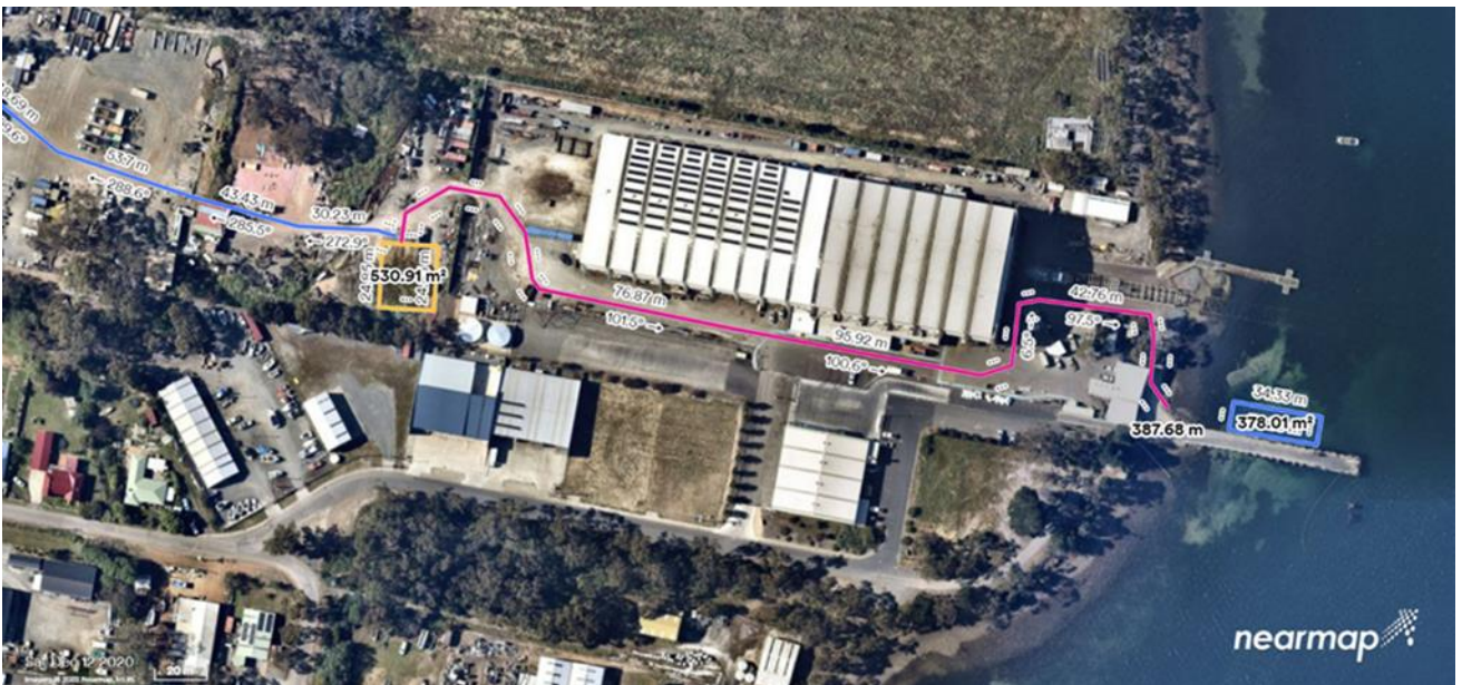
Figure 2 Secondary Contingency Loadout site at Haywards Shipyard. Truck access (Purple line) to rock stockpiling area (Yellow line). Loader route from the rock stockpile past the shipyard warehouse (Maroon line) to load the construction barge (Blue rectangle) at the Jetty
