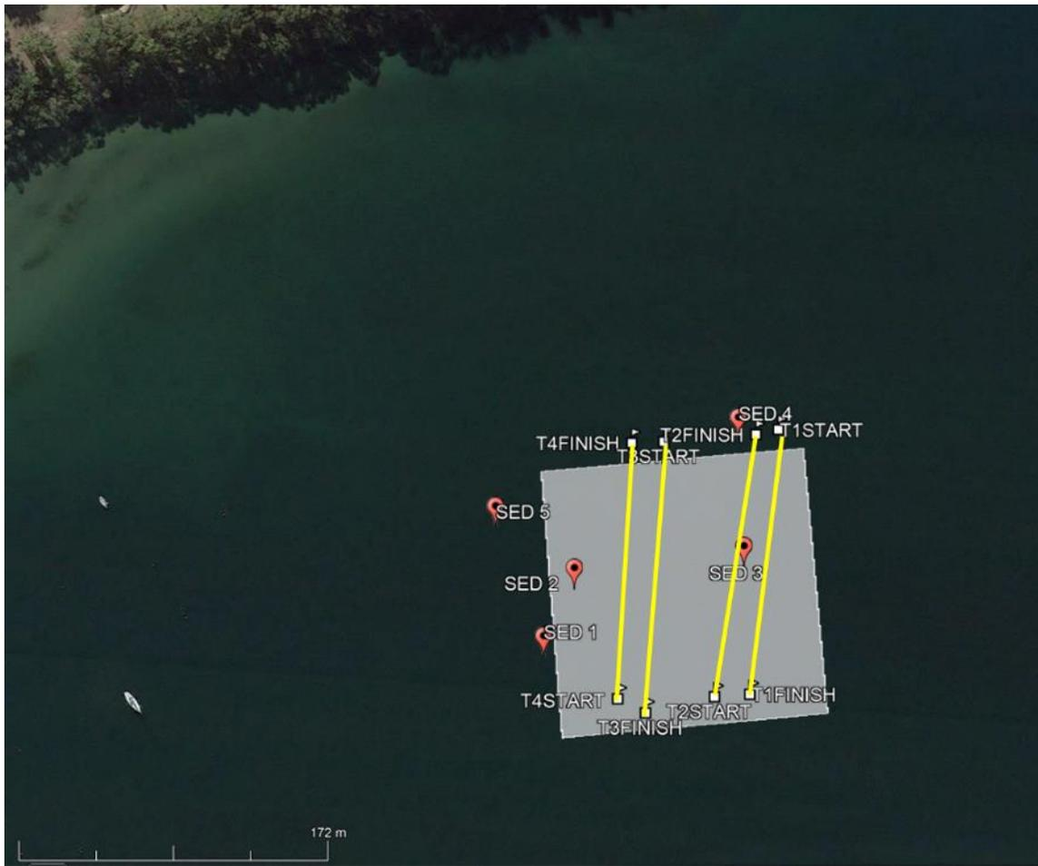
**Figure 3 Location of the dive transects (yellow) and sediment grabs (red) relative to the reef permit area at Helliwells Point, Woodbridge**
