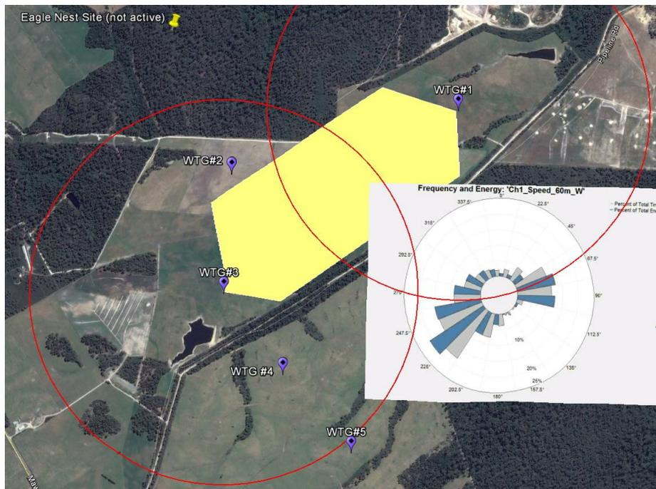
**Figure 6: Area that cannot be utilised due to wake effect considerations (shown in yellow). The red circles show an 840m radius around WTG #3 and WTG #1 and the inset wind rose shows that the predominant wind direction is south west.**
