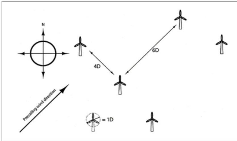
**Figure 5: Typical minimum distances between wind turbines**
