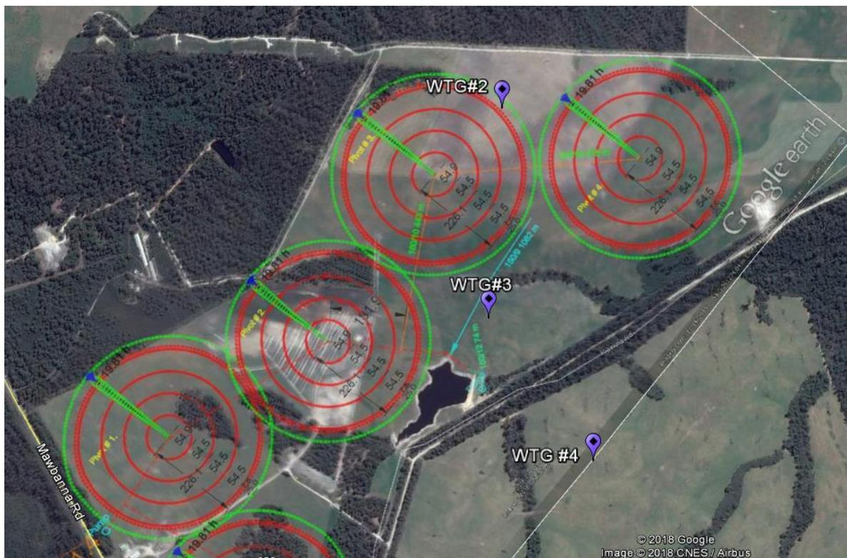
**Figure 7: Pivot irrigators restricting wind turbine placement**
