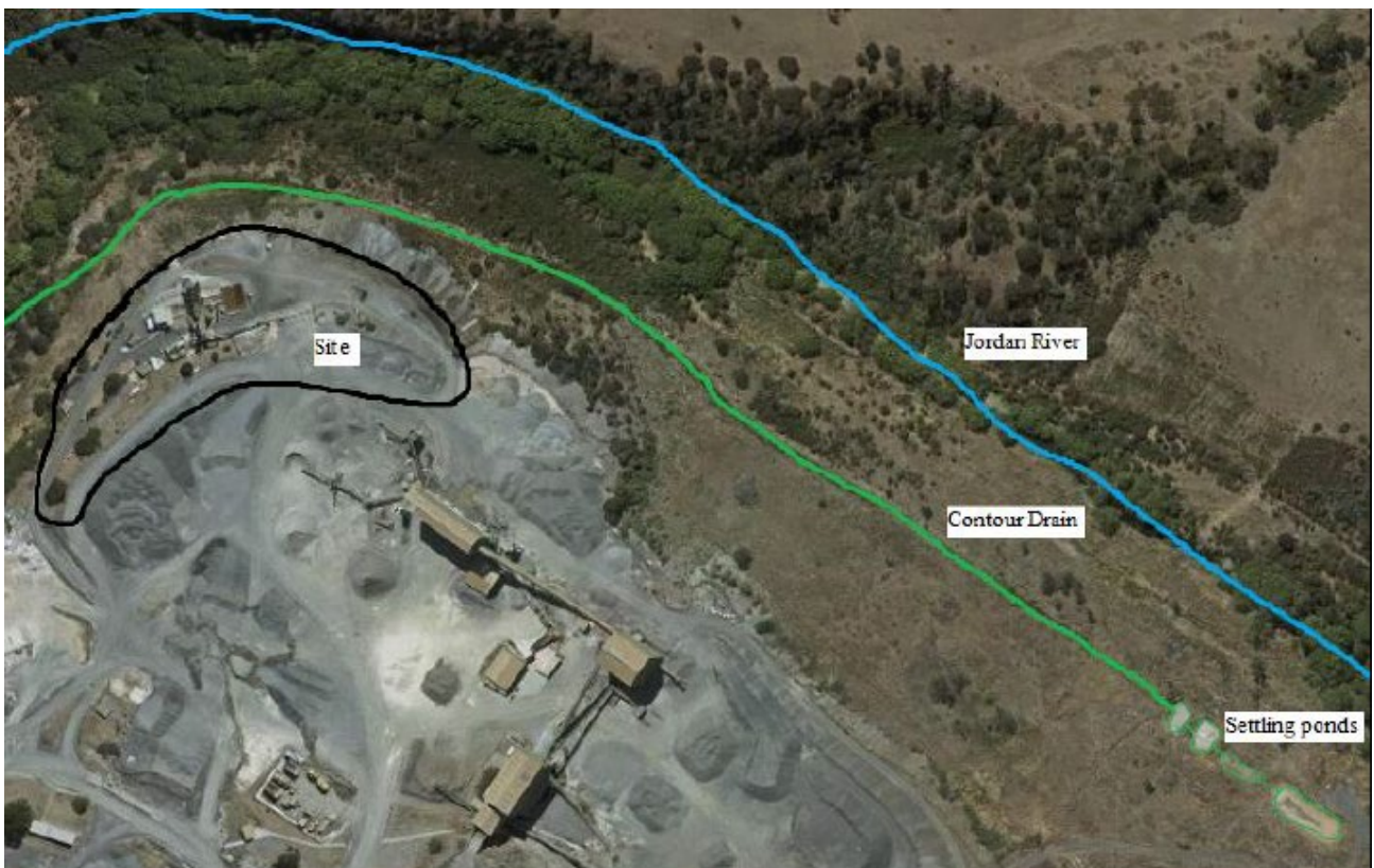
Figure 3: Bitumen plant site, and drainage features (Source: Figure 6, EER).
