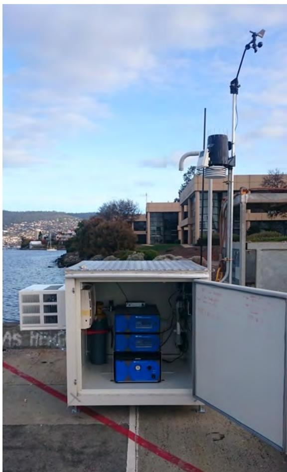
The reference-level monitoring station installed on the CSIRO wharf area includes instruments for collecting SO<sub>2</sub> ambient concentration data and weather parameters. It comprises of the Teledyne T100 UV Fluorescence SO<sub>2</sub> Analyzer, T700 gas calibration unit, Davis Vantage Pro 2 weather station and Cybertec 3G modem.
