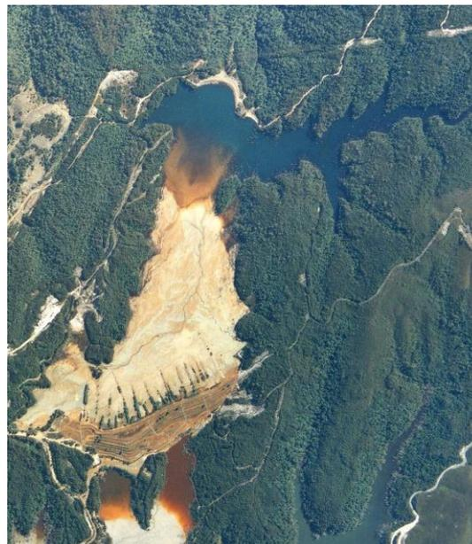
**Figure 7: Streams of iron-rich acid rock drainage seep from the Old Tailings Dam southern wall**
