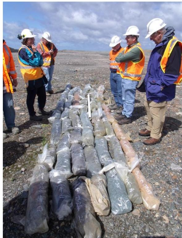
**Figure 3: Inspection of sonic bore samples B Dump (courtesy Shengjia Zeng, 2011)**
