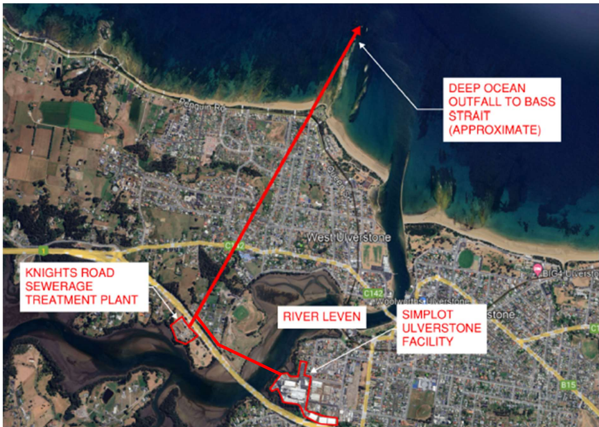
Figure 4 – General alignment of TasWater outfall pipeline
