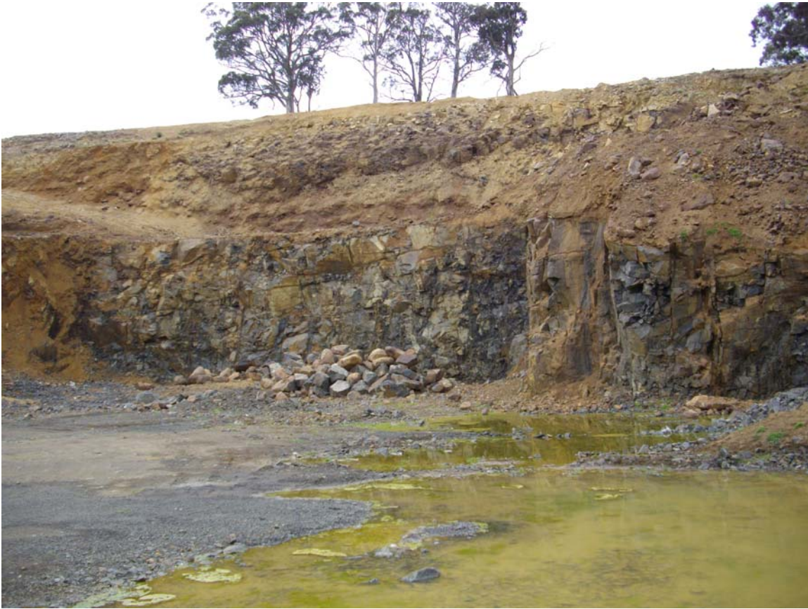
Figure 6. Dolerite high wall in the centre of the current quarry. After pre stripping approximately 0.5m of soil and regolith, the proportions of fresh and weathered dolerite are ideal for current needs and the floor level allows for control of drainage entering the quarry from the southern (right) side. Additional resource potential appears best to the southeast, i.e. obliquely to the right.
