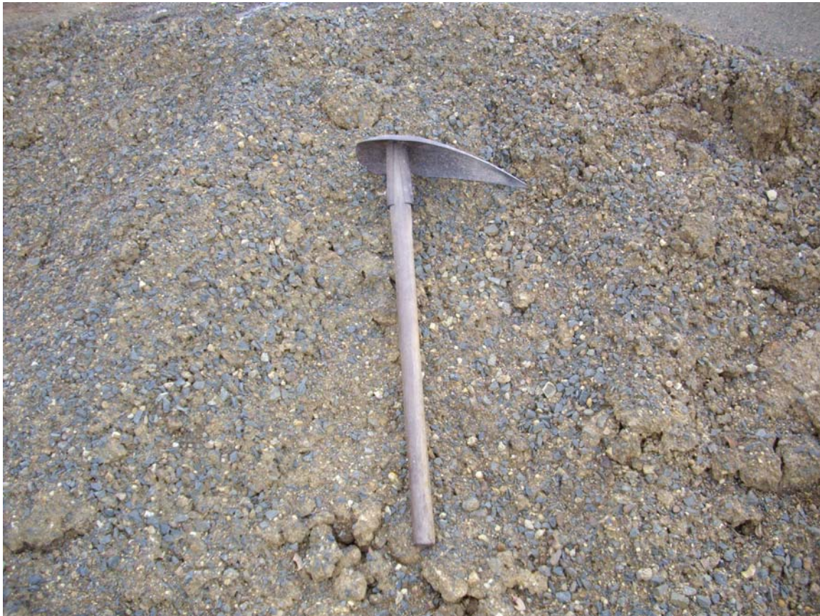
Figure 4. Aggregate for gravel road construction – approximately 70% deeply weathered dolerite and 30% fresh bluestone dolerite. Minor amounts of pale blocky hornfelsed sandstone can be tolerated.
