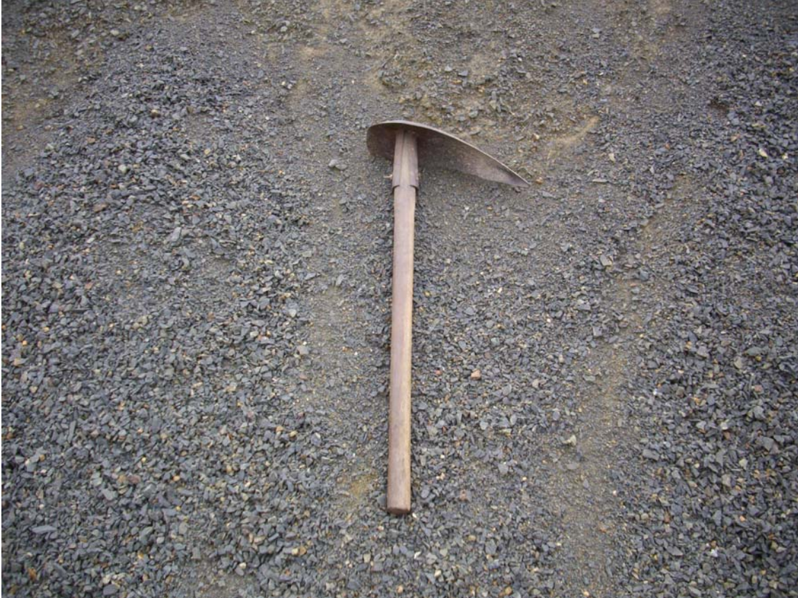
Figure 5. Aggregate for constructing the base of sealed roads – approximately 15% deeply weathered dolerite and 85% fresh bluestone dolerite. Almost none of the sedimentary rock can be tolerated.
