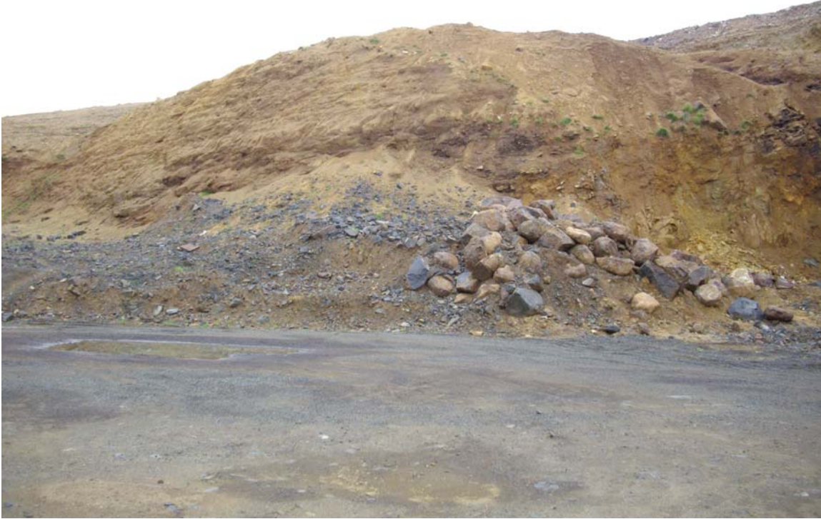
Figure 7. Northern end of the quarry, showing good quality weathered and fresh dolerite to the right, grading to increasing waste due to deeply weathered high clay dolerite and sandstone to the left (north) of photo.
