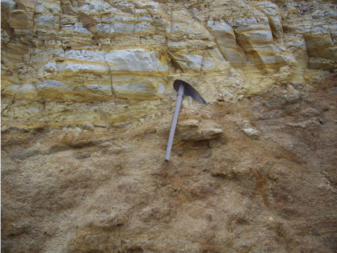
Figure 3. Shallow north dipping contact between bleached, partly silicified flat lying sandstones, overlying deeply weathered oxidized dolerite, northern end of the quarry. This dolerite is an excellent source of brown gravel for road making but the sandstone is clay rich and unstable and is generally left for rehabilitation landscaping.
