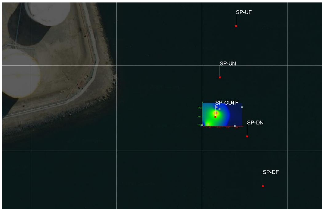
Figure 5-4 Selfs Point outfall rhodamine plume tracer results during the incoming tide (Jacobs 2016)
