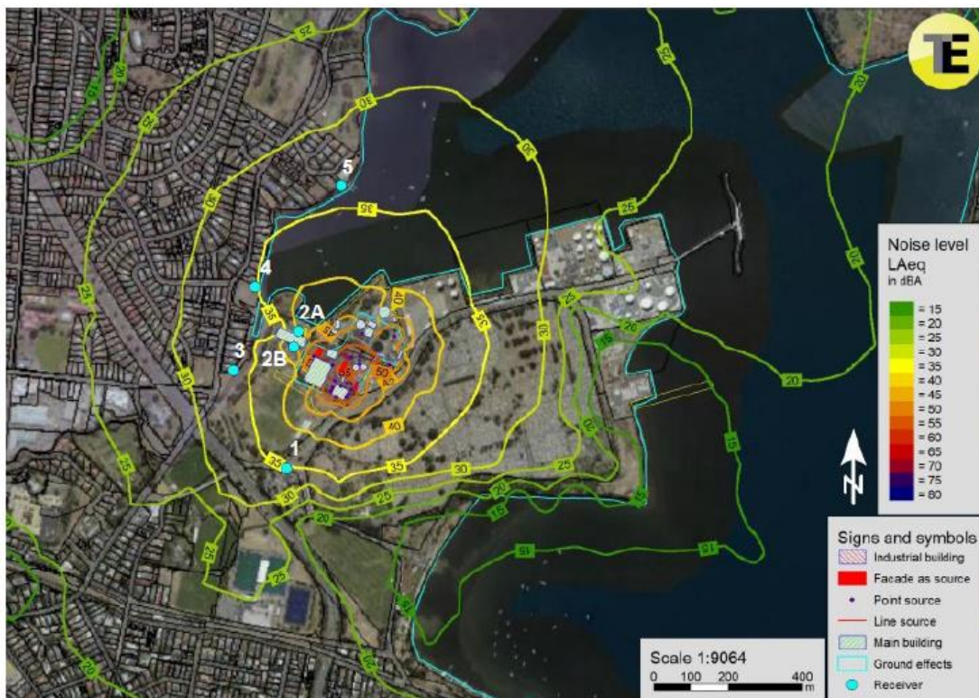
Figure 8: Predicted noise contours worst case scenario with mitigation (EIS Figure 6.10)
