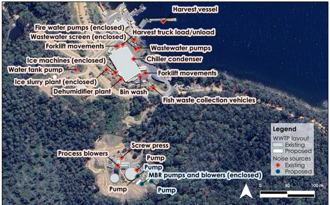
Figure 4: Markup of Noise-Generating Equipment (Source: Tassal)
