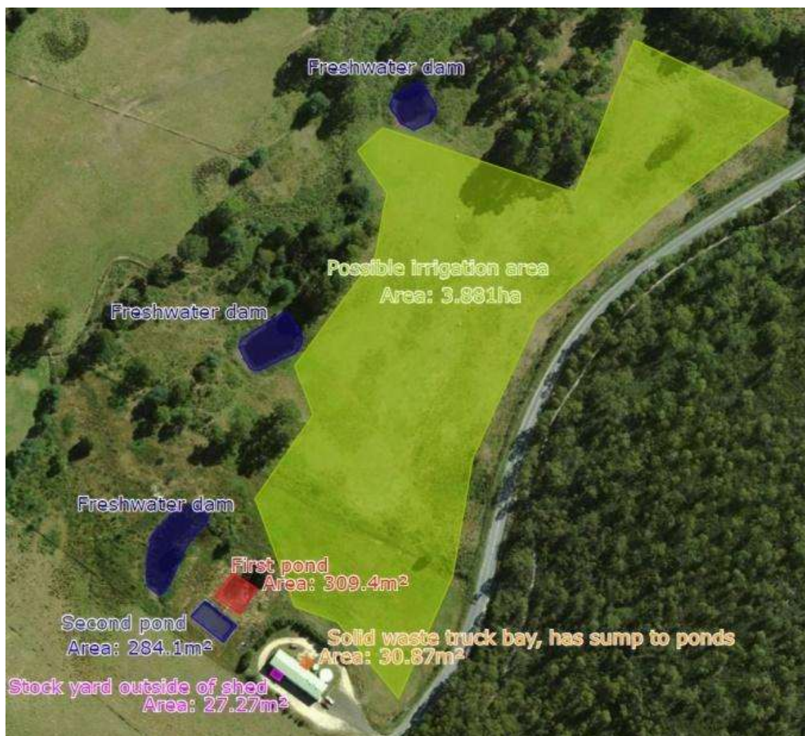
Figure 8 – Onsite infrastructure (The first pond is the only infrastructure that has the potential to emit odour). Note: solid waste includes biological waste.
