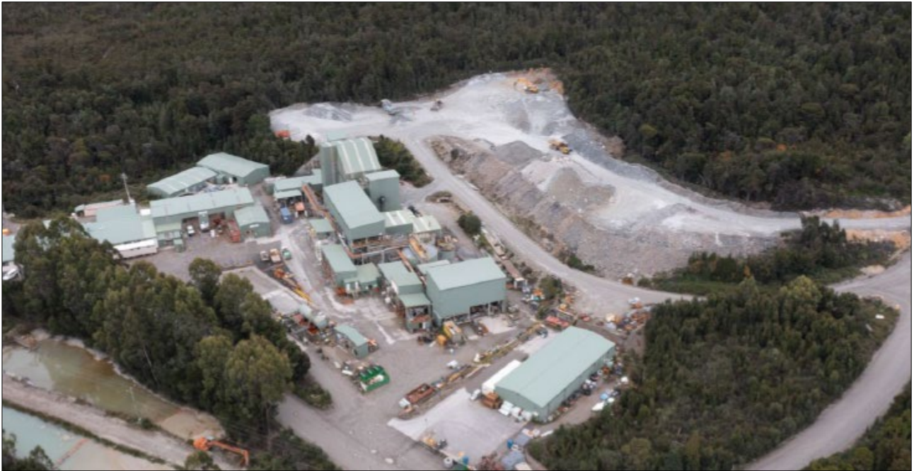
Figure 2: Henty Gold mine mill area and existing ROM pad with stockpiles (Cover image of EER)
